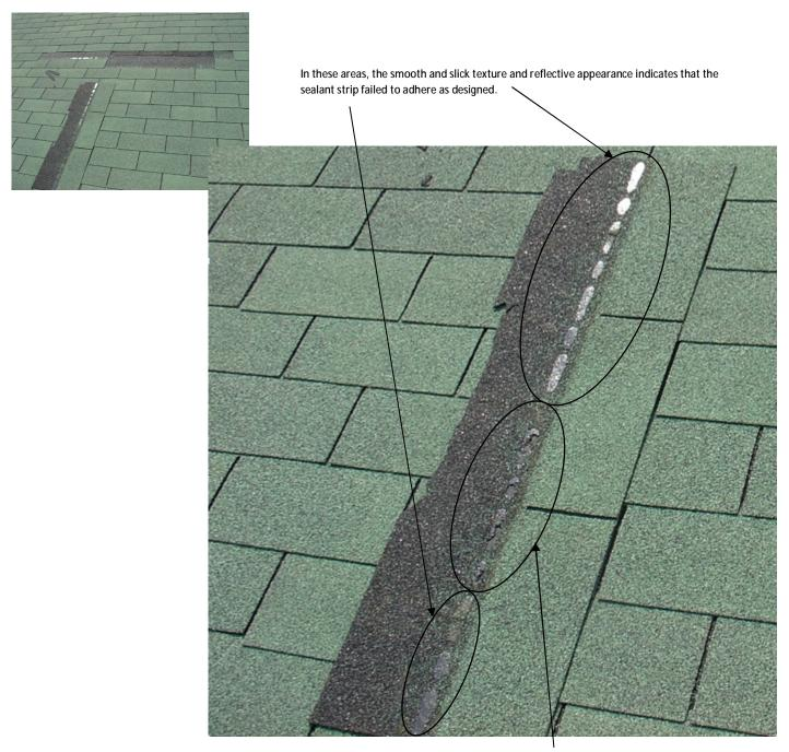
In this area, the shingle physically delaminated when it was torn from the roof by wind. This delamination indicates that, at least in this area, the shingle's sealant strip reached a design level of adhesion.
