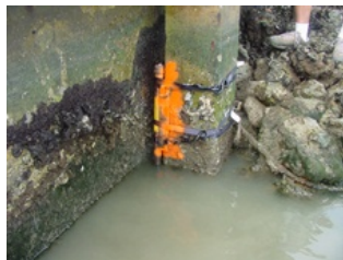
Water-level sensor deployed at WS_26A Marco Island Bayside.
