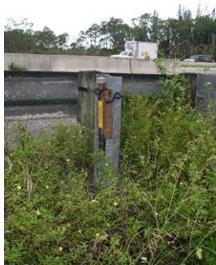
Barometric-pressure sensor deployed at WS_19 Imperial River.
