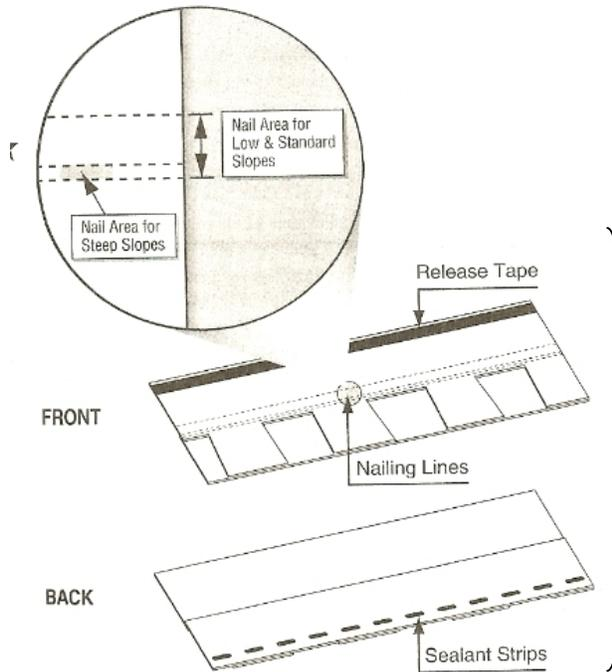
The asphalt sealant strip on many dimensional shingles is located on the backside of the shingle, near the bottom, so that when the shingles are assembled on the roof, the bottom of each overlying shingle seals to the top center of the underlying shingle.
