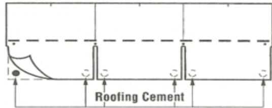
Apply 1" (25 mm) spots of asphalt roofing cement under each tab corner.
