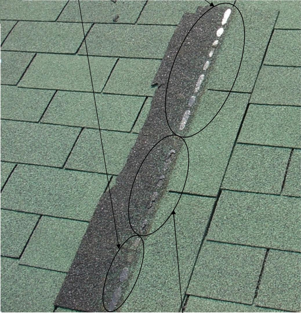
In this area, the shingle physically delaminated when it was torn from the roof by wind. This delamination indicates that, at least in this area, the shingle's sealant strip reached a design level of adhesion.
