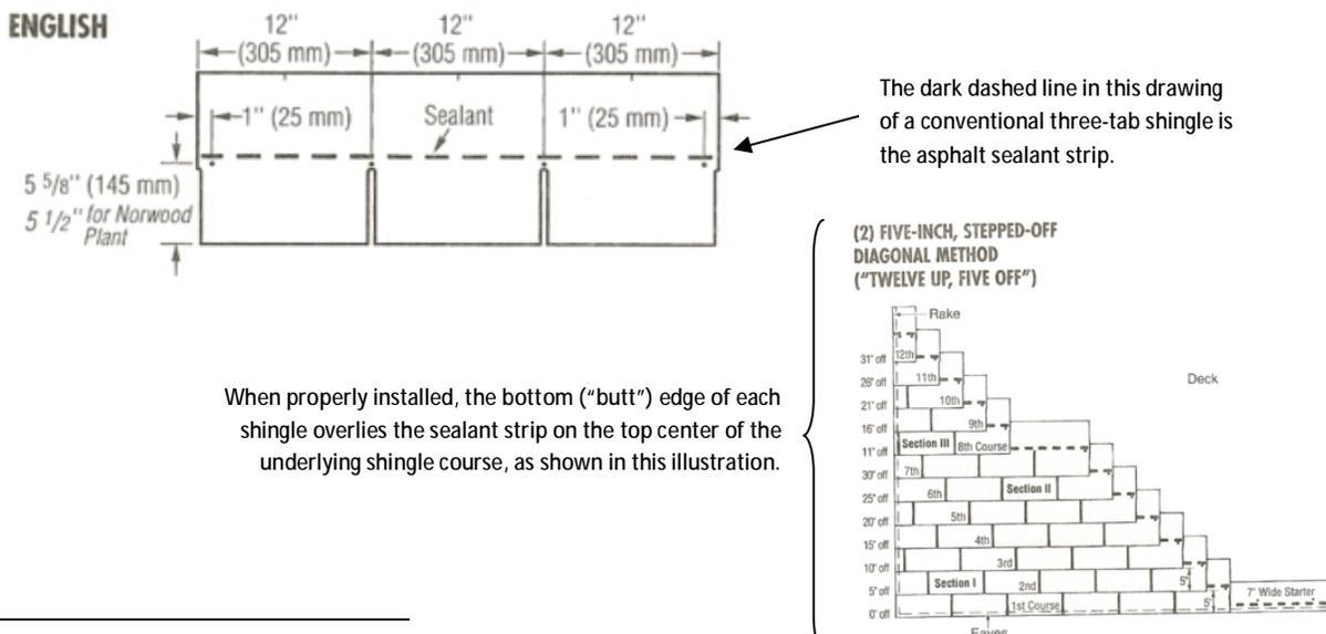
When properly installed, the bottom ("butt") edge of each shingle overlies the sealant strip on the top center of the underlying shingle course, as shown in this illustration.
